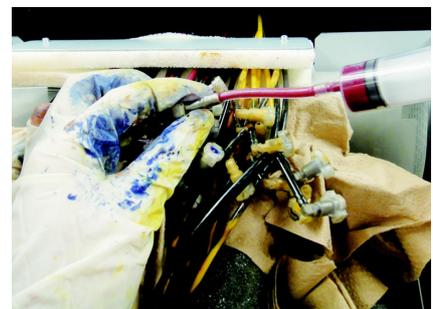
**6****Set the syringe with pressure damper to the ink port valve.**
